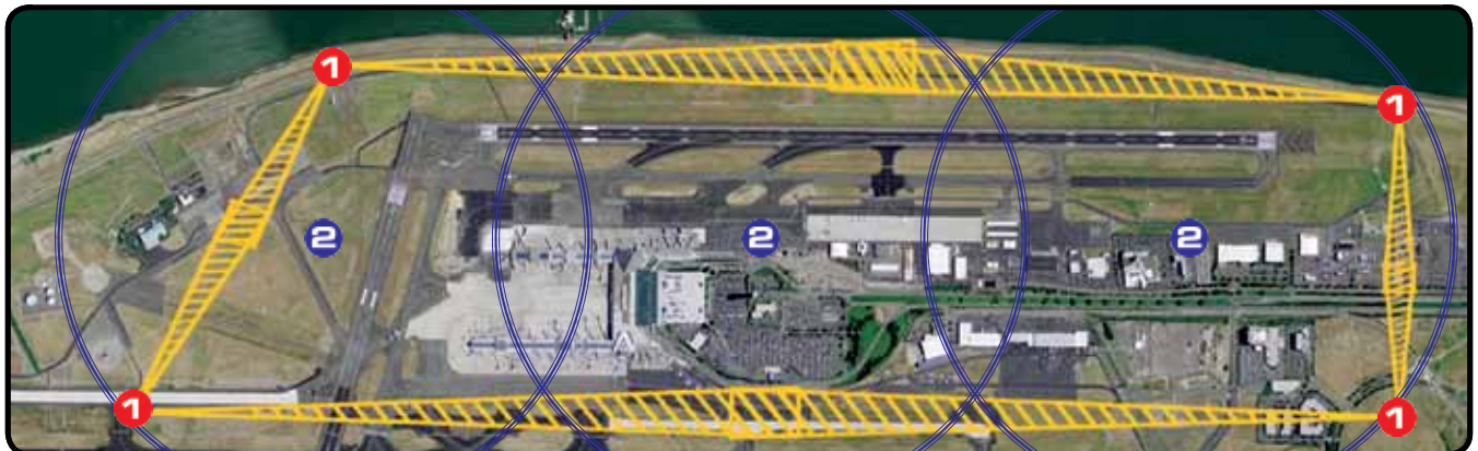
Aerial view of thermal camera layout depicting their fields of coverage and delineating the FLIR Thermal Fence perimeter.
